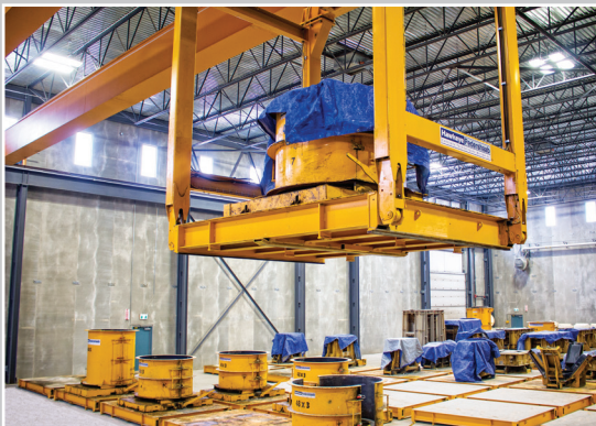
Inventory is automatically handled by an overhead manipulator
